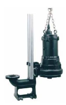
The U pump features a vortex (eddy flow) structure and wide pump casing interior, preventing clogging by waste and solid matter.
